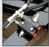
Cushion valve with 1/2" ports protects cylinders from impact loads. Preset at 2000 PSI, adjustable from 1500 - 3000 PSI
