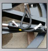
Twin 3" double acting chrome plated hydraulic cylinders for heavy duty power reversing. Located above the push frame for protection & ease of service (4" optional)
