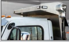
Cab shield with Built-In Tarp System
