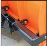
4" x 4" x 3/8" Full length structural steel tubing push frame, running gear mounts are standard
