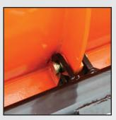
8 Moldboard-to-push frame pivot points have 1-1/4" plated pins through 1/2" ribs bolstered with second 1/2" plate bushed to 1-3/8" thick
