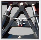
3-1/2" Steel channel A-frame supports a 1-1/2" plated king pin mounted in a 2-1/4" OD x 3/8" wall DOM tube with grease fitting
