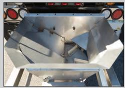
"Hex flow" chute w/24" spinner assembly for optimal spread pattern
